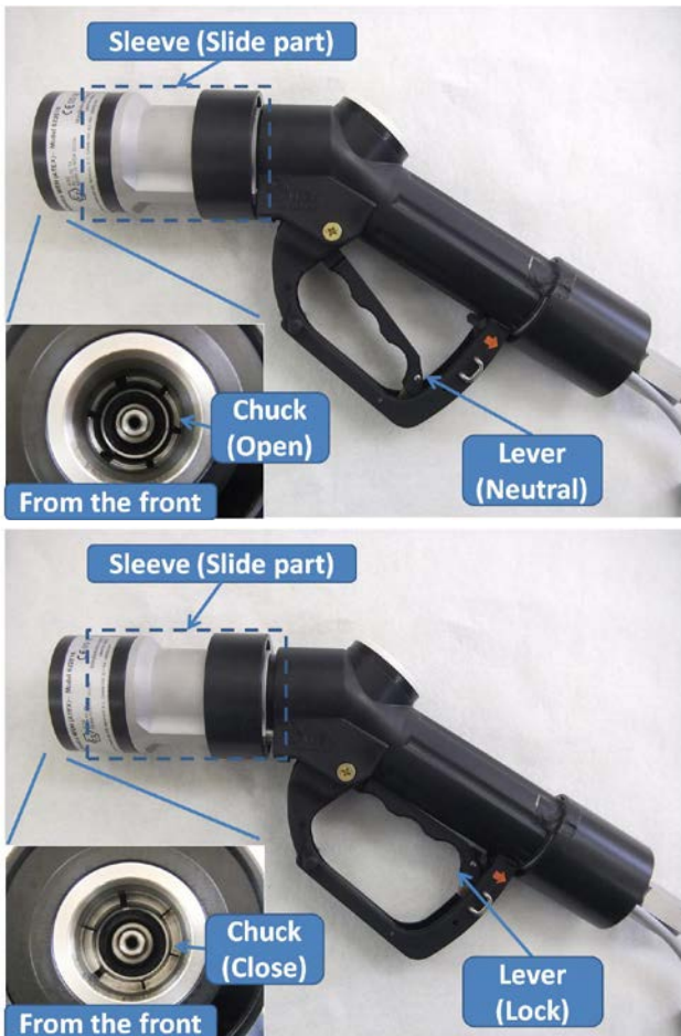
Fig. 1 Nozzle (Neutral(upper), Lock(bottom) )
