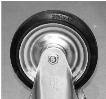
Fig. 5 Tire of robot assumed to run over human foot
