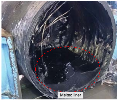
Fig. 10 Melted liner of the cylinder
